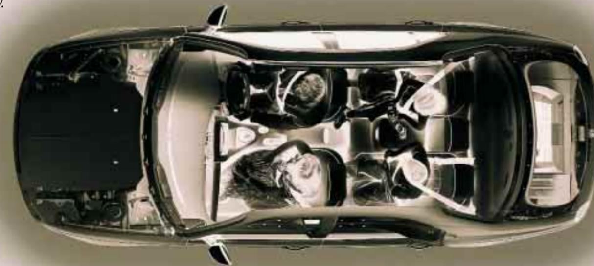
By contrast, the second line of defence is a reinforced passenger cell designed to protect the occupants and the fuel tank by retaining its shape. Side impacts are fended off by stiffened, anti-jam door structures with diagonal reinforced beams, interlinked through the chassis to share stresses over a wide area.
